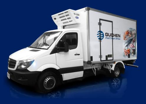
Guchen Thermo integrated standby units are with the scroll electric compressor inside the condenser units, that can be plug into external AC power supply when truck engine stops. Saving Fuel/ Saving Money/ Eco-friendly. The compact and integrated structure are light-weight, low noise, low failure rate, easy for installation and maintenance!
